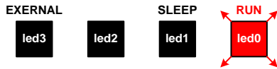
With PWM signals present on LI and HI, the RUN LED is blinking
