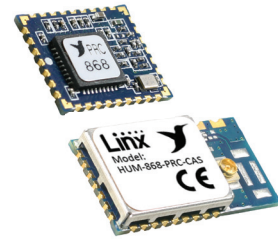
Figure 9: Standard (top) and Pre-certified (bottom) HumPRC™ Modules
