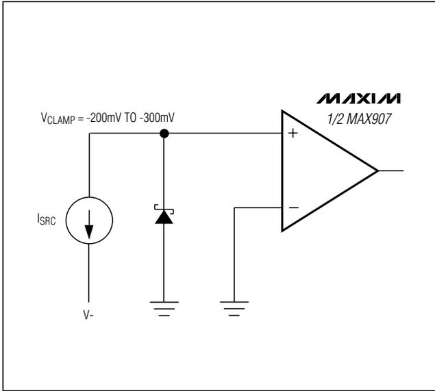
Figure 3. Schottky Clamp for Input Driven Below Ground
