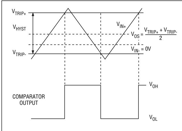
Figure 1. Input and Output Waveforms, Noninverting Input Varied
