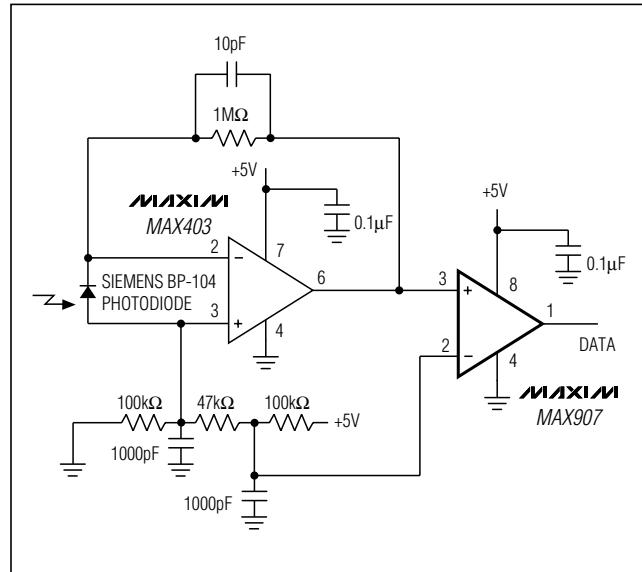
Figure 4. Battery-Operated Infrared Data Link Consumes Only 1mA
