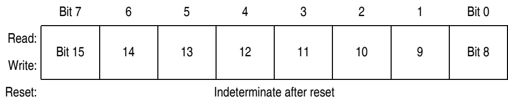
Figure 12-14. TIMB Channel 0 Register High (TBCH0H)
