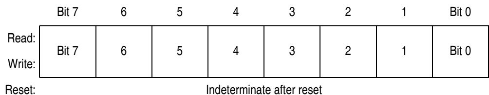
Figure 12-15. TIMB Channel 0 Register Low (TBCH0L)
