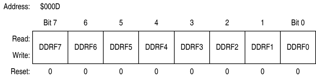
Figure 17-19. Data Direction Register F (DDRF)
