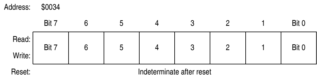
Figure 12-19. TIMB Channel 2 Register Low (TBCH2L)
