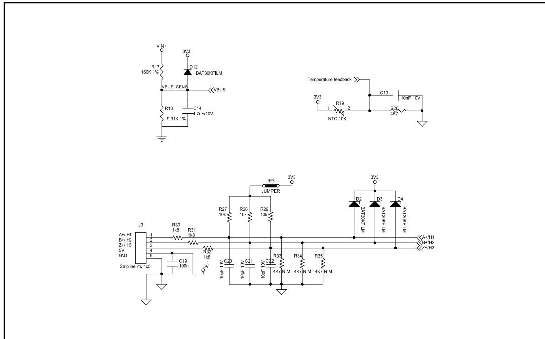
**Figure 5: Schematic - Analog conditioning and Current protection circuit**
