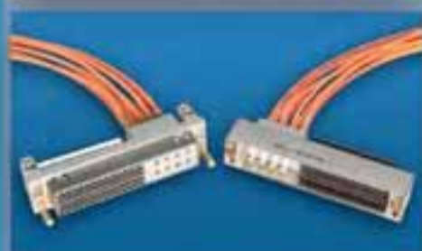
Hybrid LRM Interconnects with Brush Contacts and MIL-PRF-29504 Fiber Optic Termini
