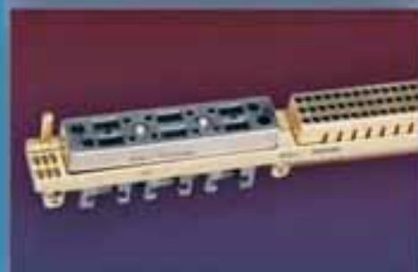
LRM (Line Replaceable Modules) with MT Fiber Optic Ferrules
