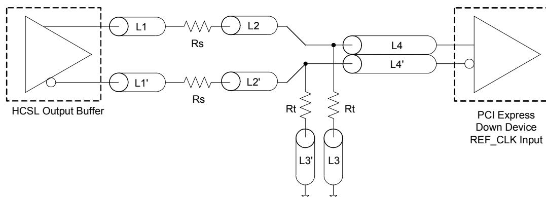
Figure 2: PCI Express Connector Routing
