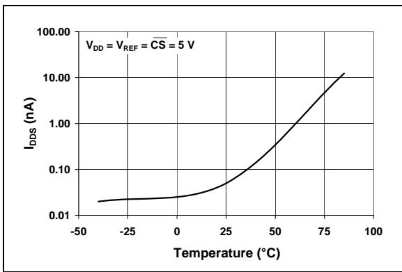
**FIGURE 2-38:**  $I_{DSS}$  vs. Temperature.
