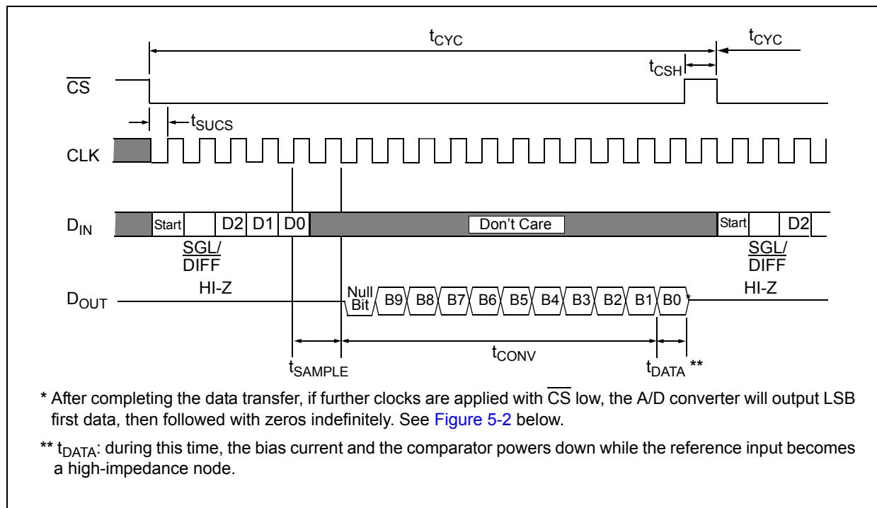
**FIGURE 5-1:** Communication with the MCP3004 or MCP3008.
