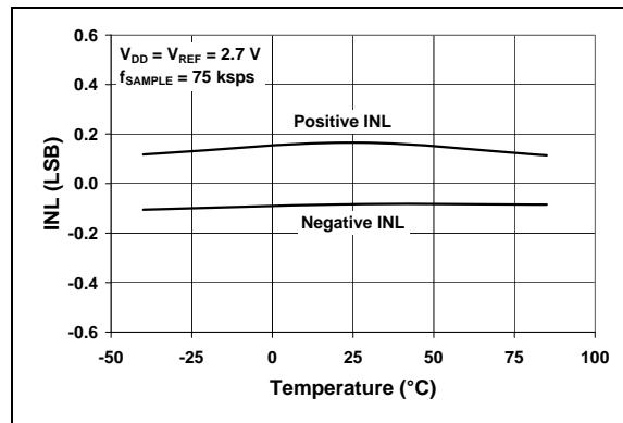
**FIGURE 2-10:** Integral Nonlinearity (INL) vs. Temperature ( $V_{DD} = 2.7V$ ).
