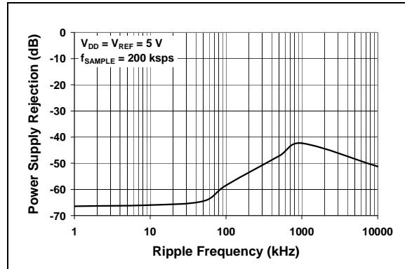
**FIGURE 2-29:** Power Supply Rejection (PSR) vs. Ripple Frequency.
