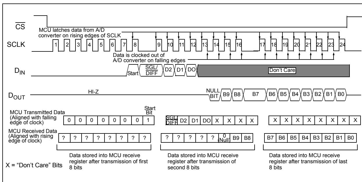
**FIGURE 6-1:** SPI Communication with the MCP3004/3008 using 8-bit segments
