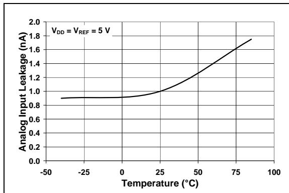
**FIGURE 2-39:** Analog Input Leakage Current vs. Temperature.
