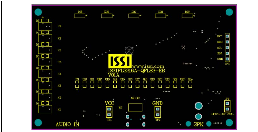
Figure 4: Board Component Placement Guide - Top Layer
