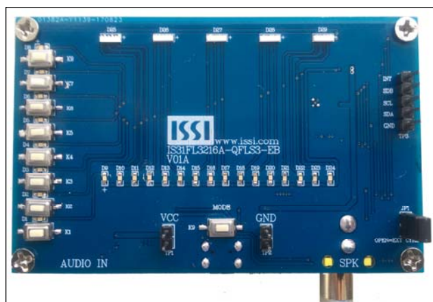
Figure 1: Photo of IS31FL3216A Evaluation Board
