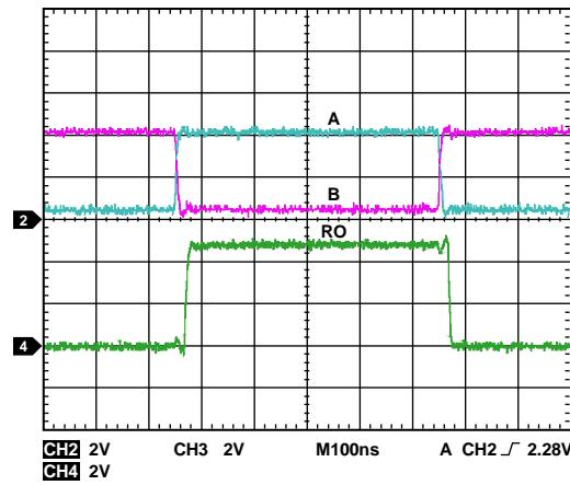
Figure 10. Receiver Output
