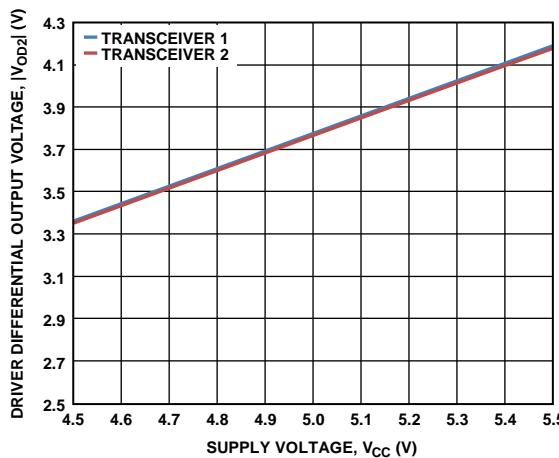
Figure 7. Driver Differential Output Voltage vs. Supply Voltage
