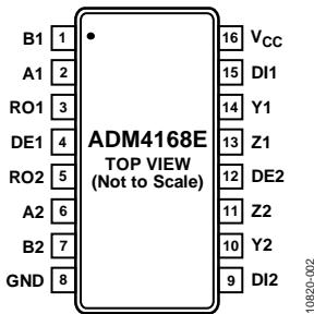
Figure 2. Pin Configuration
