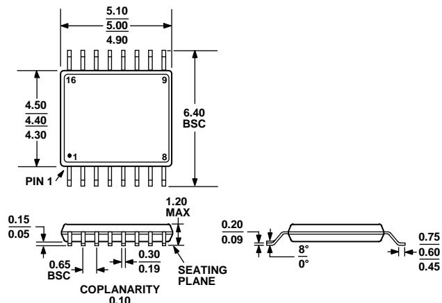
**Figure 17. 16-Lead Thin Shrink Small Outline Package [TSSOP]**
