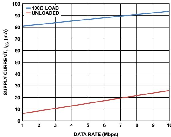
Figure 6. Supply Current vs. Data Rate
