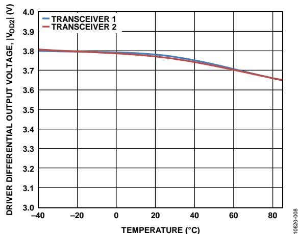
Figure 4. Driver Differential Output Voltage vs. Temperature
