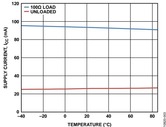
Figure 3. Supply Current vs. Temperature, Data Rate = 10 Mbps
