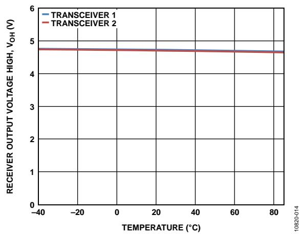
Figure 5. Receiver Output Voltage High vs. Temperature
