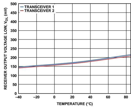
Figure 8. Receiver Output Voltage Low vs. Temperature
