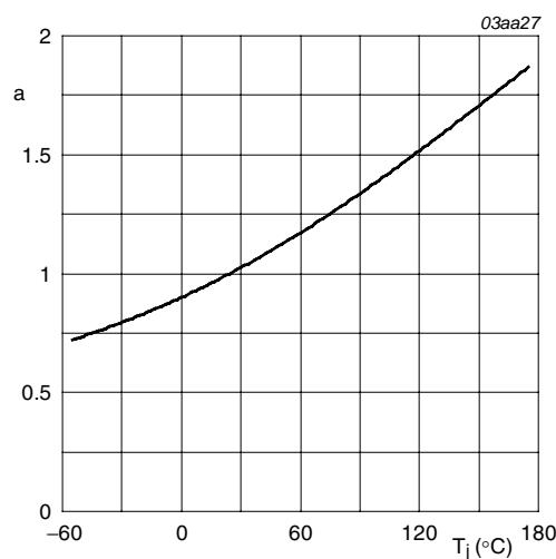
$$a = \frac{R_{DSon}}{R_{DSon}(25^\circ\text{C})}$$
