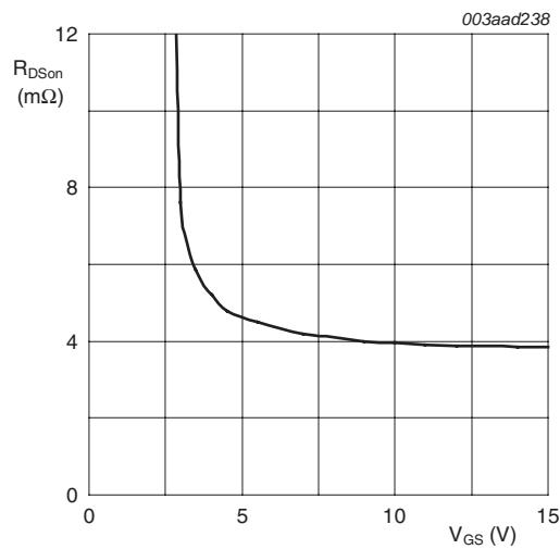
$T_j = 25^\circ\text{C}; I_D = 15 \text{ A}$
