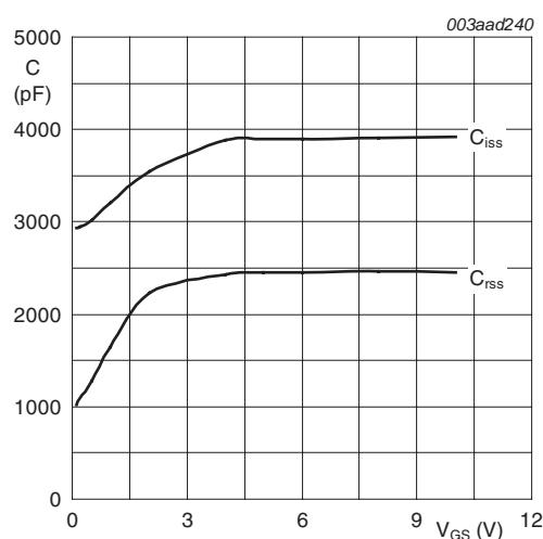
$V_{DS} = 0 \text{ V}; f = 1 \text{ MHz}$
