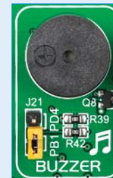
Figure 18-2: Use jumper J21 to connect Piezo buzzer on PB1 or PD4 pin
