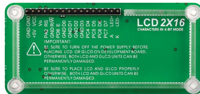
Figure 10-1: On-board LCD 2x16 display connector
