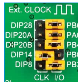
Figure 4-9: Position of the jumpers for DIP14
