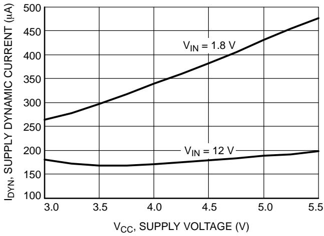
Figure 8. Supply Dynamic Current vs. Supply Voltage
