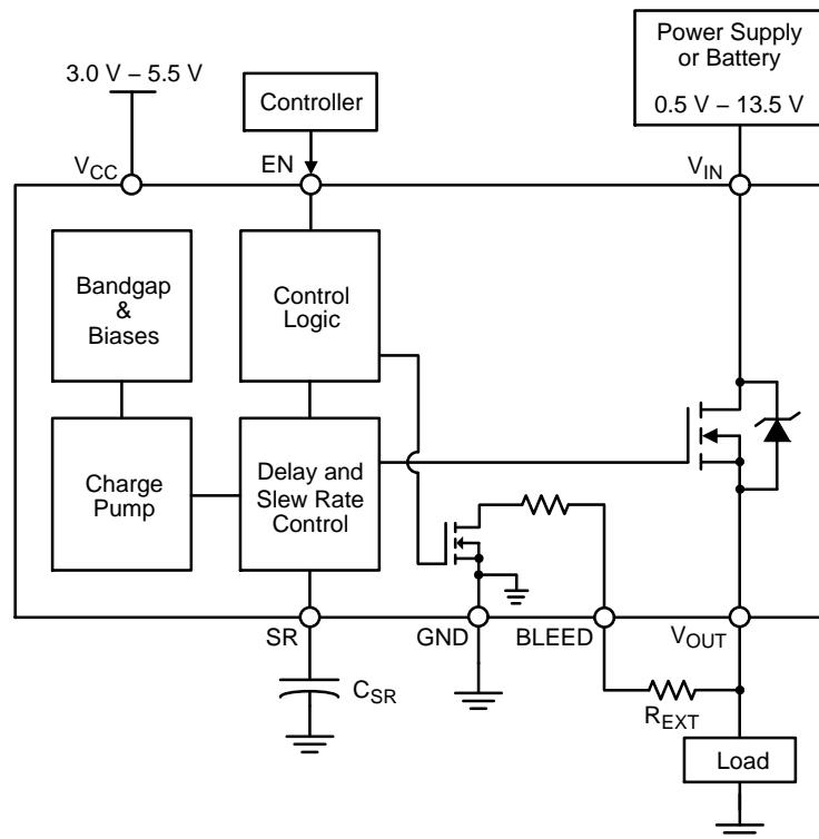
Figure 30. NCP45525 Typical Application Diagram – Load Switch
