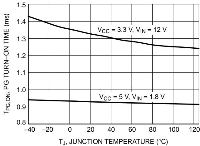
Figure 24. Power Good Turn-on Time vs. Temperature
