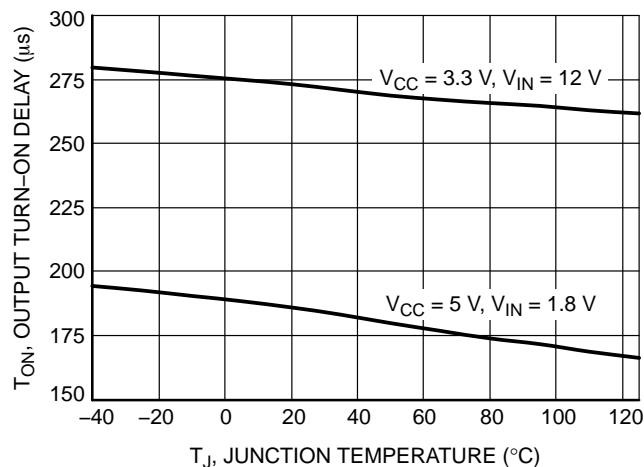
Figure 20. Output Turn-on Delay vs.
