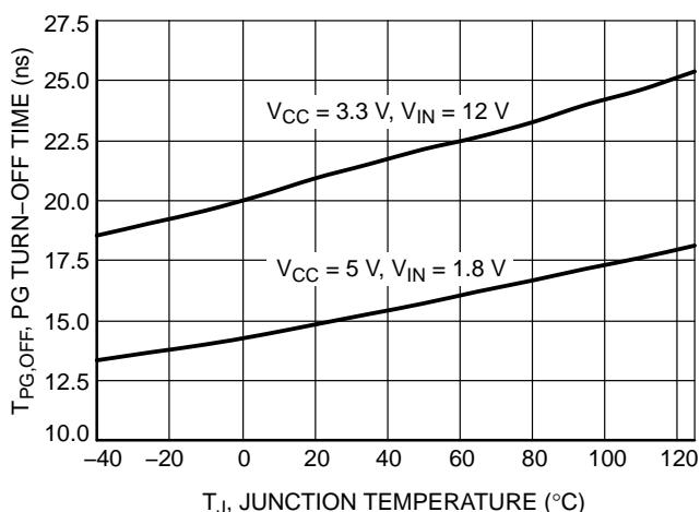
Figure 26. Power Good Turn-off Time vs. Temperature
