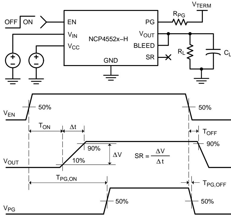
**Figure 2. Switching Characteristics Test Circuit and Timing Diagram**
