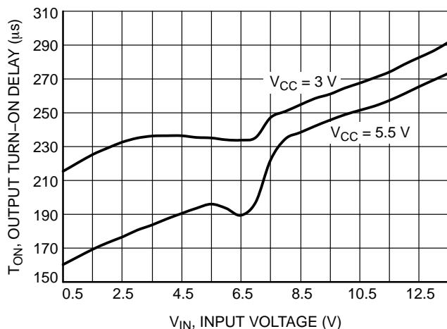
Figure 19. Output Turn-on Delay vs. Input
