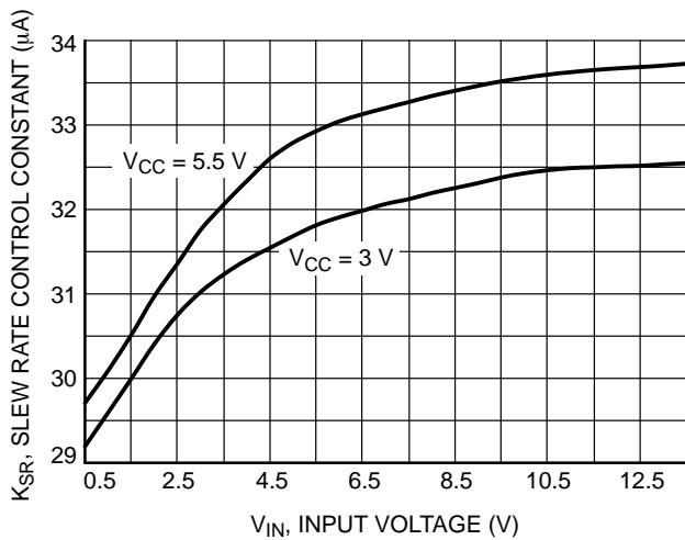
Figure 15. Slew Rate Control Constant vs.
