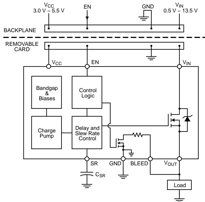
Figure 31. NCP45525 Typical Application Diagram – Hot Swap
