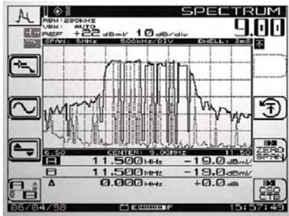
Reverse digital modem signal
