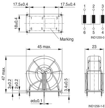
Part tolerances to ISO 2768-cL / ISO 8015. Size ISO 14405 (E) All dimensions in mm
