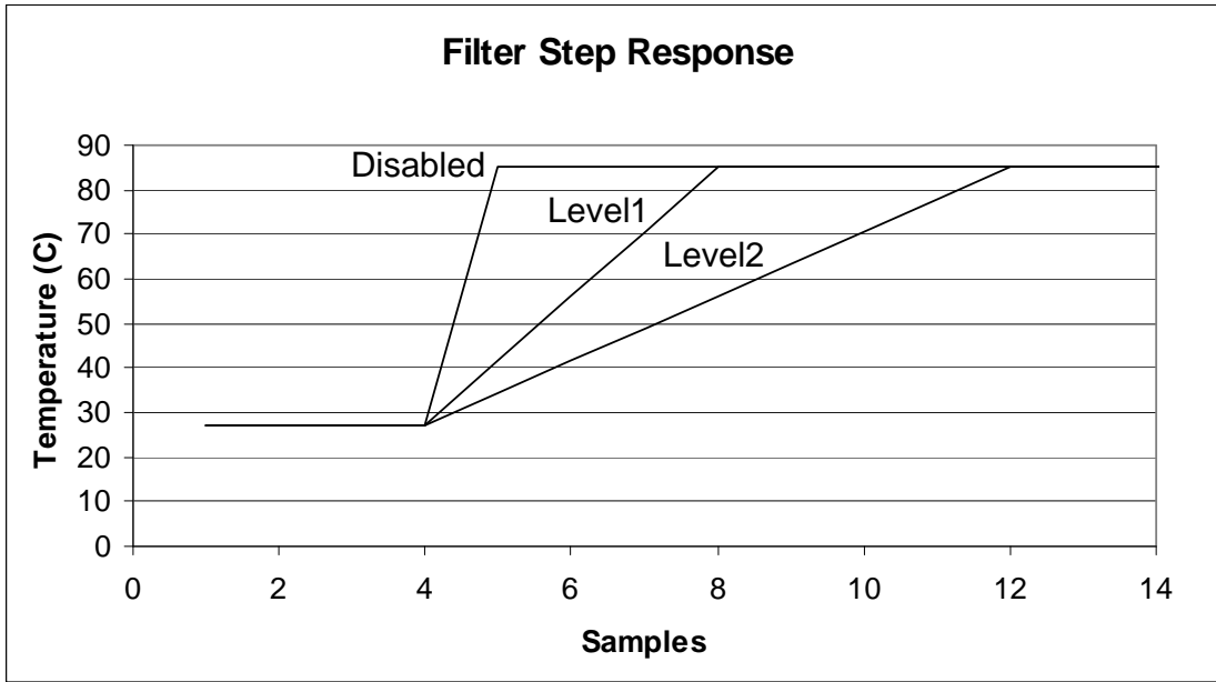
Figure 5.4 Temperature Filter Step Response
