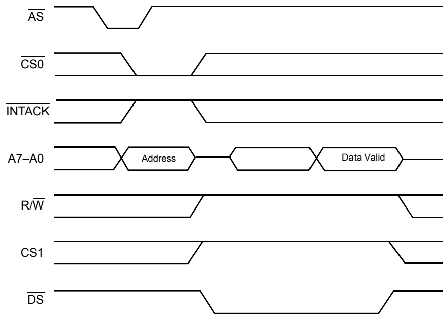
Figure 18. Z80230 Read Cycle Timing
