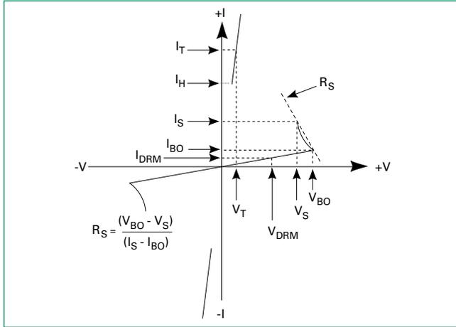
**Figure 2: On-state Current vs. On-state Voltage (Typical)**
