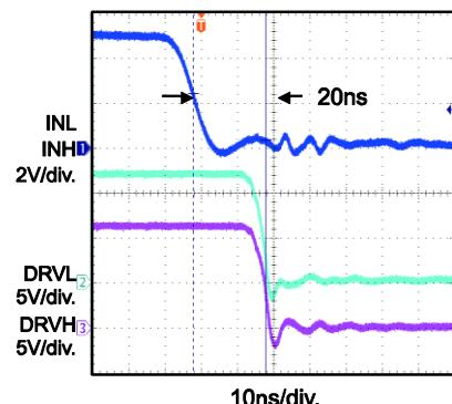
**Gate Drive Matching  $T_{MOFF}$**
