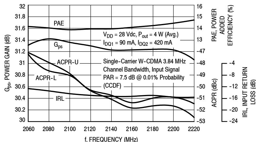
**Figure 5. Power Gain, Input Return Loss, Power Added Efficiency and ACPR versus Frequency @  $P_{\text{out}} = 4$  Watts Avg.**
