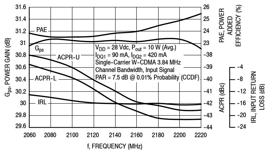
**Figure 6. Power Gain, Input Return Loss, Power Added Efficiency and ACPR versus Frequency @  $P_{\text{out}} = 10$  Watts Avg.**
