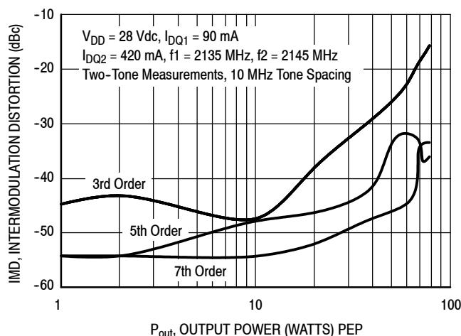
**Figure 11. Intermodulation Distortion Products versus Output Power**
