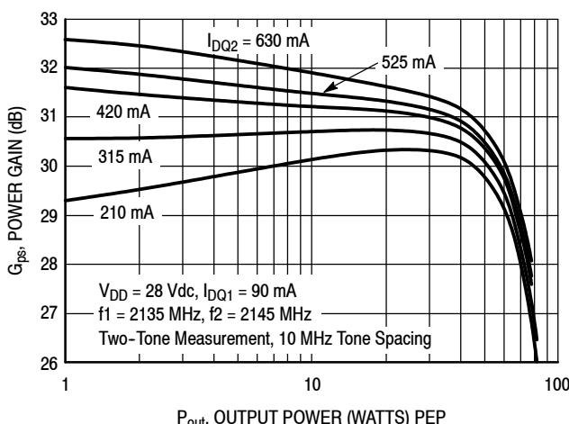
**Figure 7. Two-Tone Power Gain versus Output Power @  $I_{\text{DQ1}} = 90$  mA**
