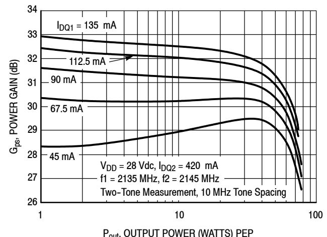
**Figure 8. Two-Tone Power Gain versus Output Power @  $I_{\text{DQ2}} = 420$  mA**
