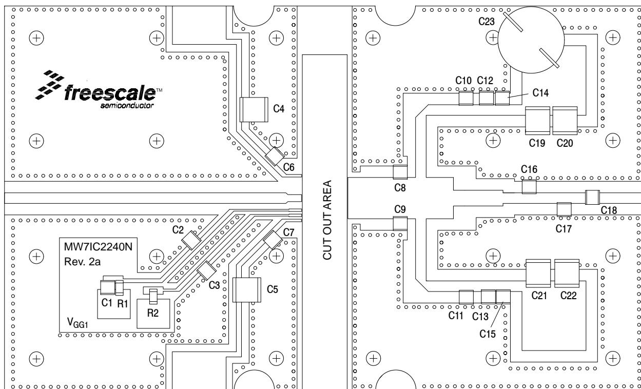
Figure 4. MW7IC2240NR1(GNR1)(NBR1) Test Circuit Component Layout
