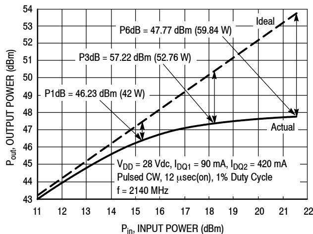
**Figure 13. Pulsed CW Output Power versus Input Power**
