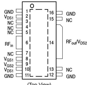
Note: Exposed backside of the package is the source terminal for the transistors.
