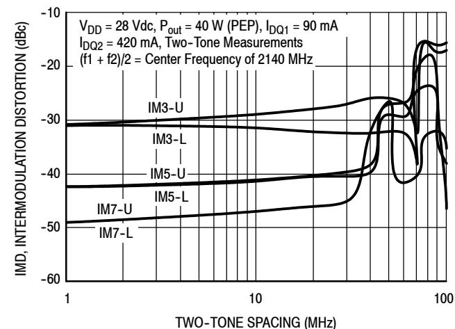
**Figure 12. Intermodulation Distortion Products versus Tone Spacing**
