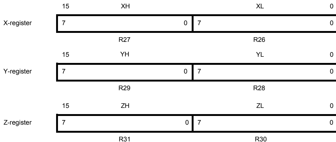
Figure 8-3. The X-, Y-, and Z-registers
