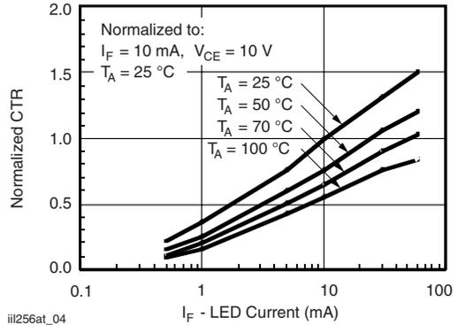
Figure 4. Normalized CTR vs.  $I_F$  and  $T_{amb}$
