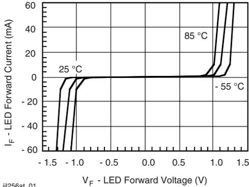
Figure 1. LED Forward Current vs. Forward Voltage
