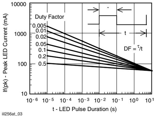
Figure 3. Peak LED Current vs. Duty Factor,  $\tau$
