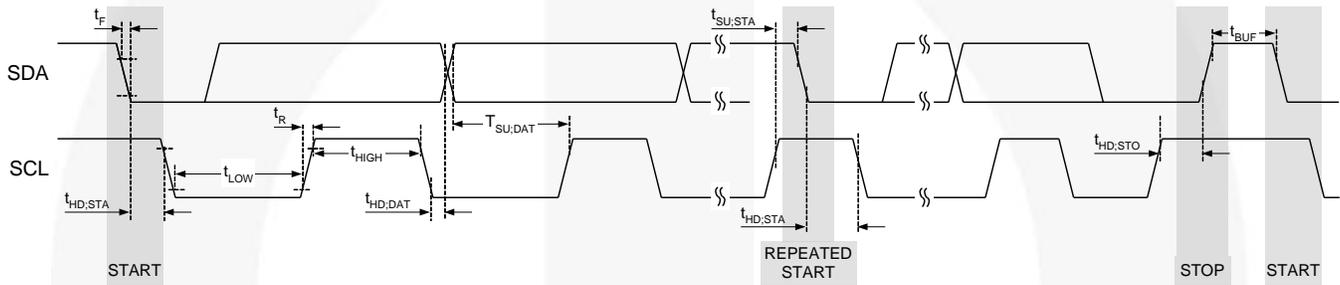
Figure 4. I<sup>2</sup>C Interface Timing for Fast and Slow Modes
