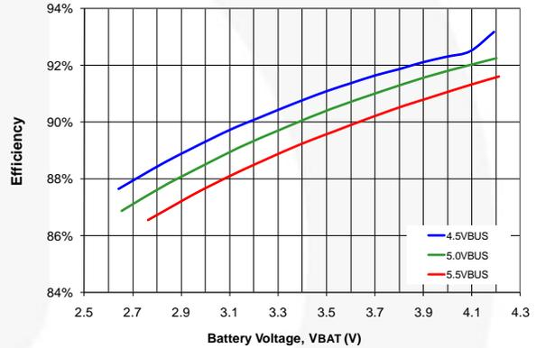
Figure 9. Charger Efficiency vs.  $V_{BUS}$ ,  $I_{INLIM}=500\text{ mA}$
