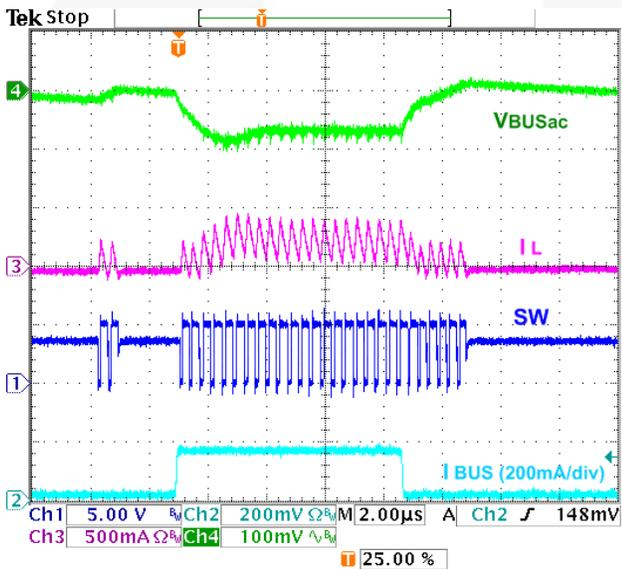
Figure 31. Load Transient, 5-155-5 mA,  $t_R=t_F=100\text{ ns}$
