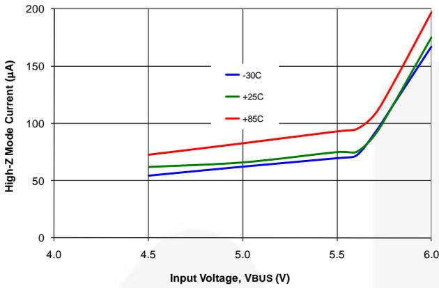
Figure 16. V<sub>BUS</sub> Current in High-Impedance Mode with Battery Open
