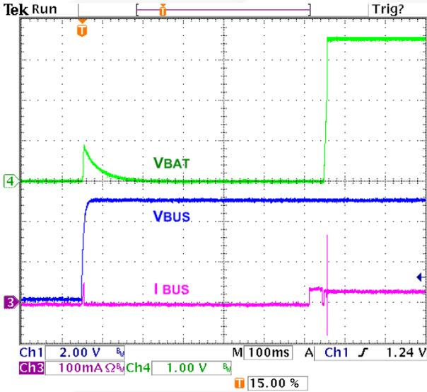
Figure 18. No Battery, V<sub>BUS</sub> at Power Up
