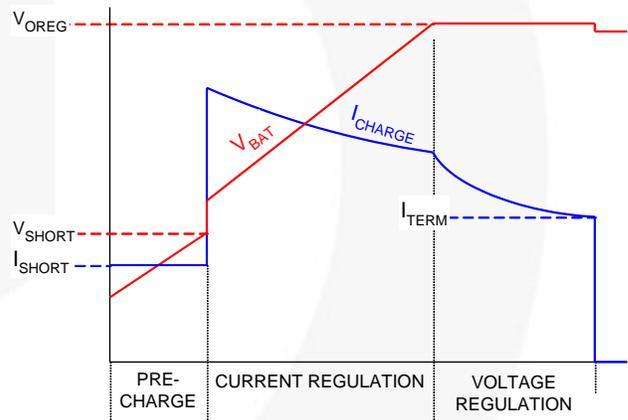
Figure 34. Charge Curve, I<sub>INLIM</sub> Limits I<sub>CHARGE</sub>
