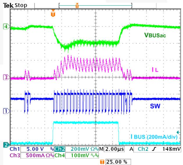
Figure 32. Load Transient, 5-255-5 mA,  $t_R=t_F=100\text{ ns}$
