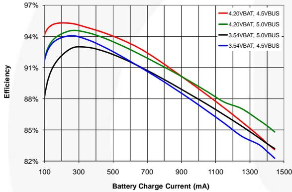
Figure 8. Charger Efficiency, No  $I_{INLIM}$ ,  $I_{CHARGE}=1450\text{ mA}$
