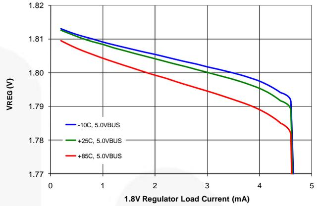
Figure 17. V<sub>REG</sub> 1.8 V Output Regulation
