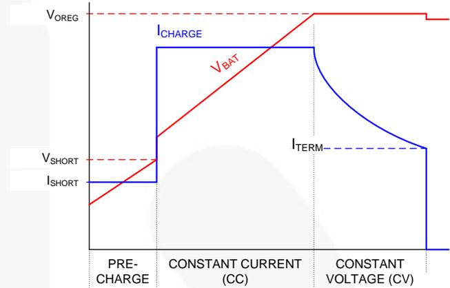
Figure 33. Charge Curve, I<sub>CHARGE</sub> Not Limited by I<sub>INLIM</sub>
