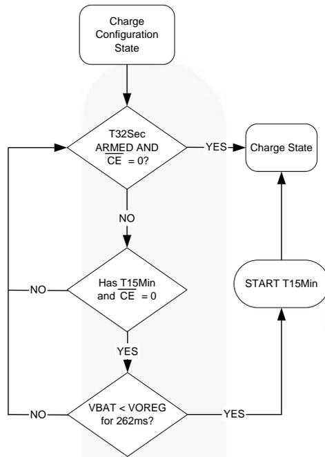
**Figure 37. Charge Configuration**
