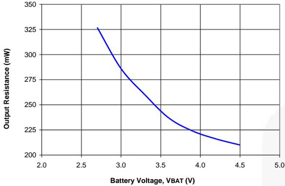
**Figure 40. Output Resistance (R<sub>OUT</sub>)**
