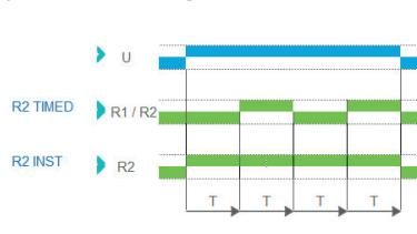
Function Di - Symmetrical flashing (ON Start)
