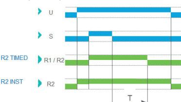
Function D - Symmetrical flashing (OFF Start)
