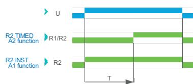
Function Ac - On/Off Delay (Delay on make/break)
