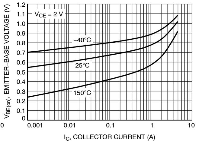
Figure 7.  $V_{BE(on)}$  Voltage
