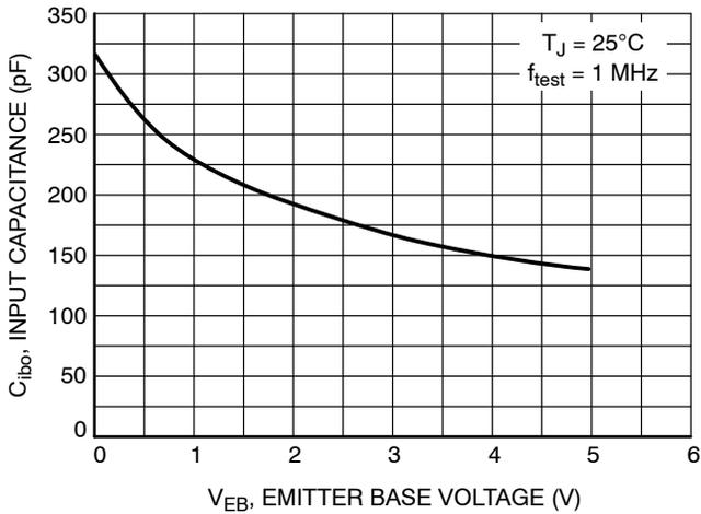
Figure 10. Input Capacitance
