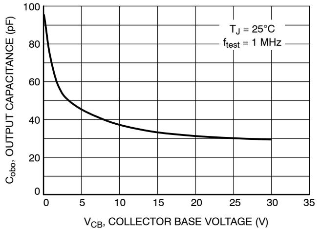
Figure 11. Output Capacitance
