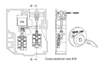
(6) Operation Key removed, solenoid ON, and trapped key removed.
