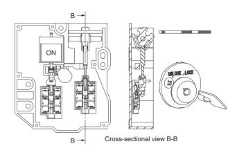
(3) Operation Key inserted, solenoid OFF, and trapped key inserted. Status: Door locked and trapped key cannot be removed.
