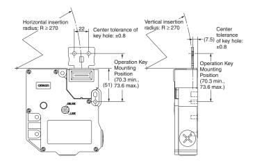
D4JL+D4JL-K2 (with Front-inserted Operation Key)
