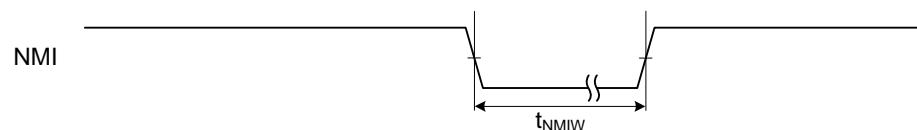
**Figure 5.6 NMI Interrupt Input Timing**
