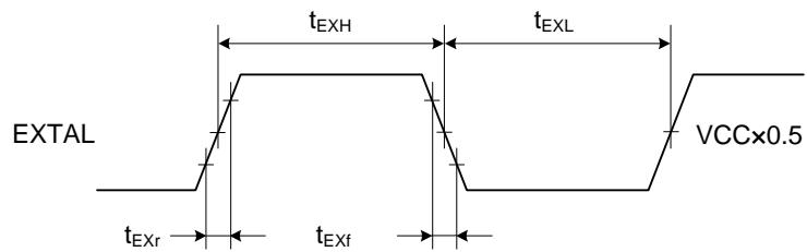
Figure 5.4 EXTAL External Input Clock Timing
