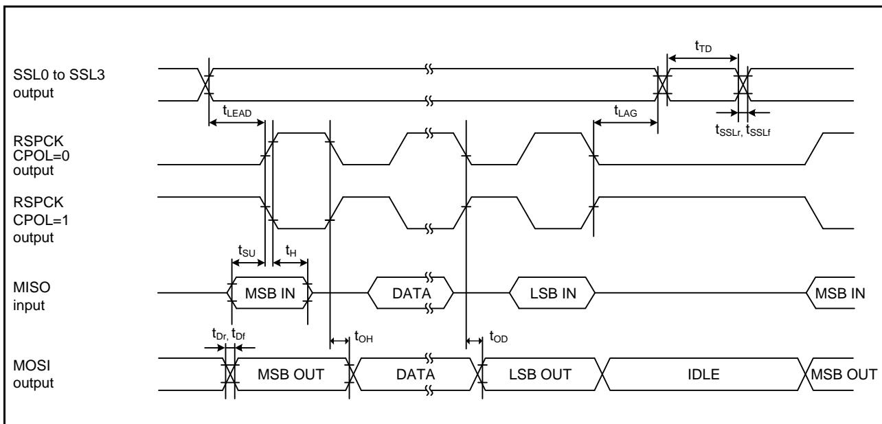
Figure 5.12 RSPI Timing (Master, CPHA = 0)
