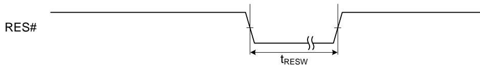
**Figure 5.5 Reset Input Timing**
