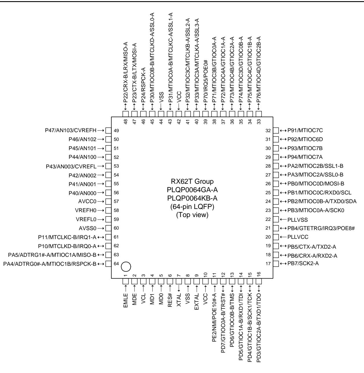
Figure 1.7 Pin Assignment of the 64-Pin LQFP
