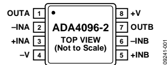
Figure 1. 8-Lead, MSOP (RM-8), ADA4096-2
