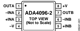
Figure 1. 8-Lead, MSOP (RM-8), ADA4096-2
