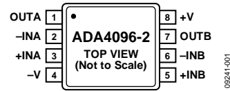
Figure 1. 8-Lead, MSOP (RM-8), ADA4096-2
