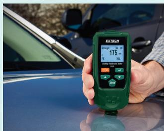
**Dual technology provides automatic recognition for ferrous and non-ferrous substrates without having you guess the material. Allows for quick, one-handed operation for non-destructive measurement of the coating thickness on various surfaces.**
