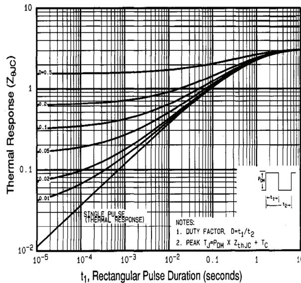
Fig. 11 - Maximum Effective Transient Thermal Impedance, Junction-to-Case
