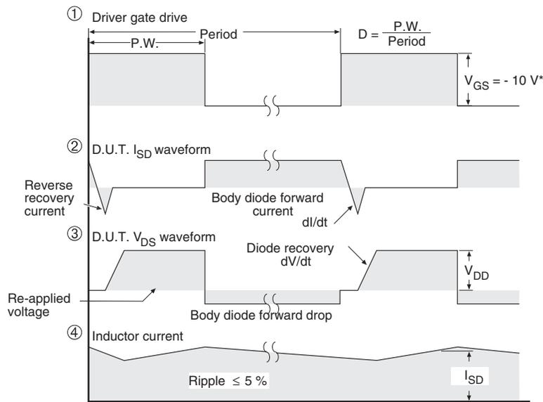
\*  $V_{GS} = -5V$  for logic level and  $-3V$  drive devices
