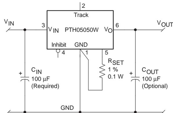
**Figure 5.  $V_O$  Adjust Resistor Placement**
