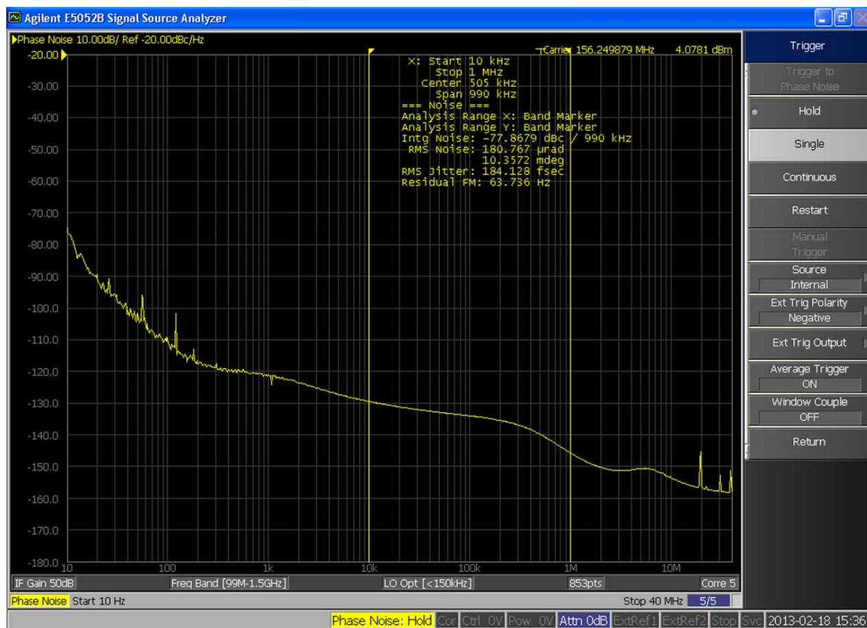
Figure 1. Si535/536 Typical Phase Noise at 156.25 MHz
