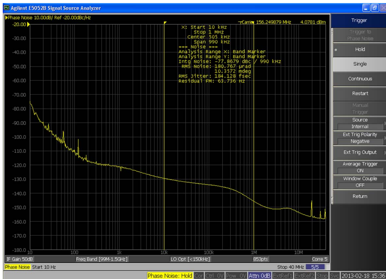
Figure 1. Si535/536 Typical Phase Noise at 156.25 MHz
