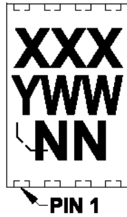
8-Lead TDFN (2x3x0.75 mm)(MCP6V32)
