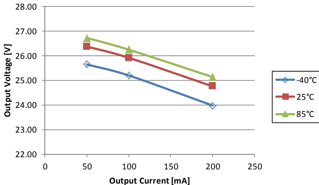
Fig. 4 Output Characteristics with V<sub>IN</sub>=15V
