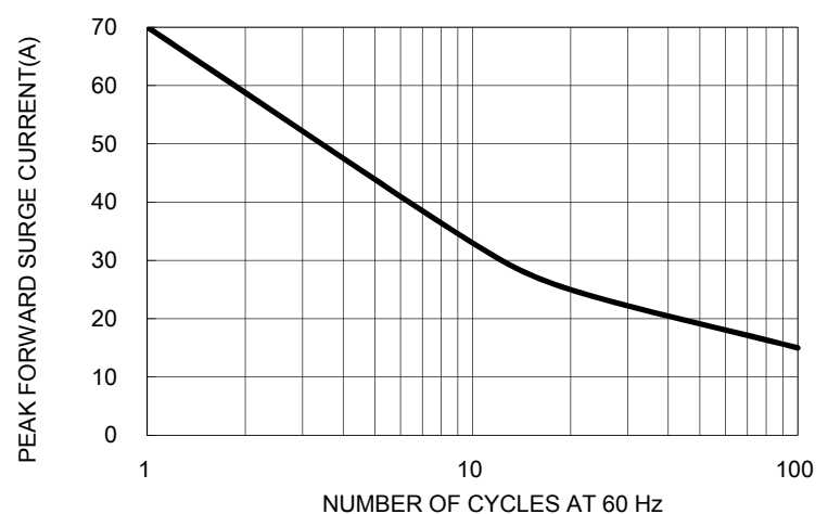
FIG. 2 MAXIMUM FORWARD SURGE CURRENT
