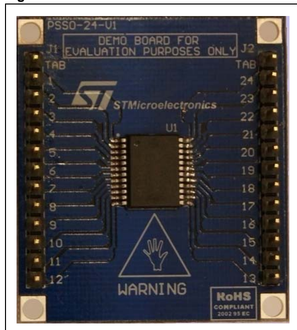
Figure 1. VND5E025AK evaluation board
