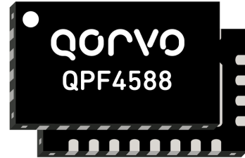
24 Pin 5x3 mm QFN Package
