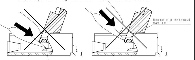
2. The actuator rotates around the rotational axis as shown below. Rotate the actuator.
