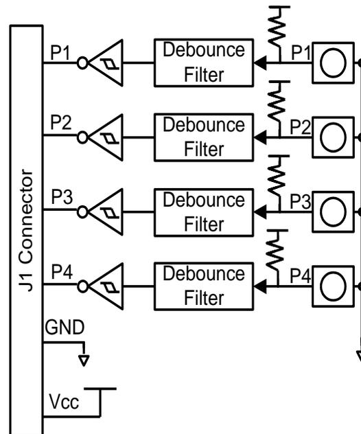
Figure 1. BTN circuit diagram.
