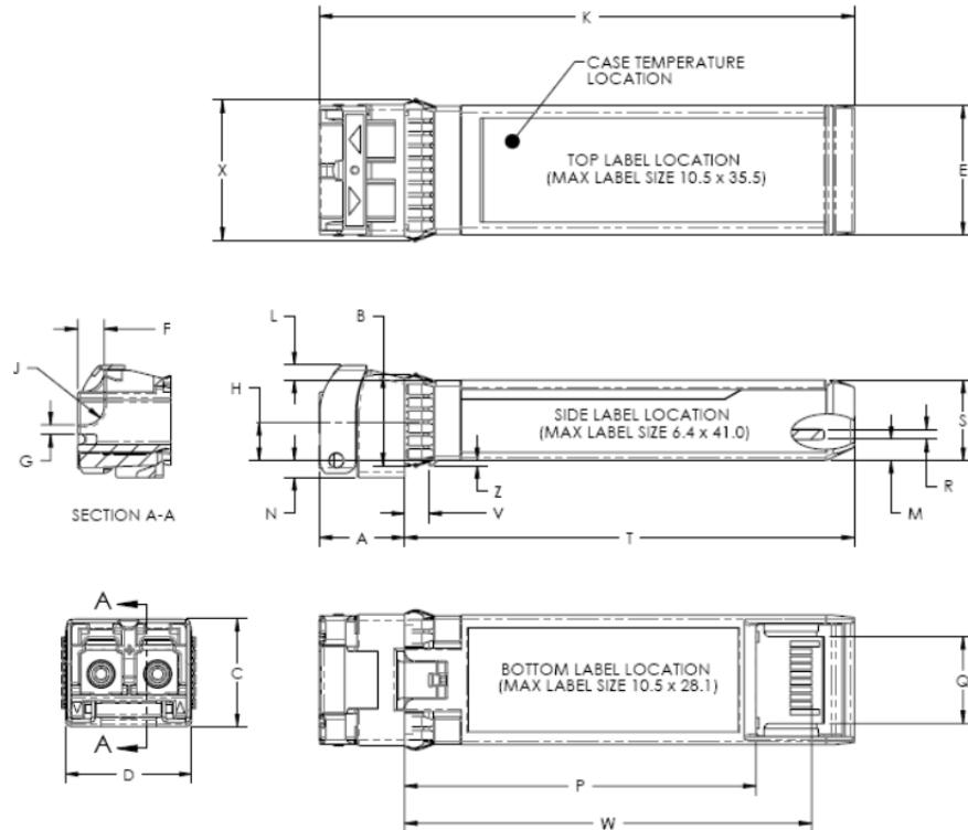
Figure 2. Mechanical Dimensions
