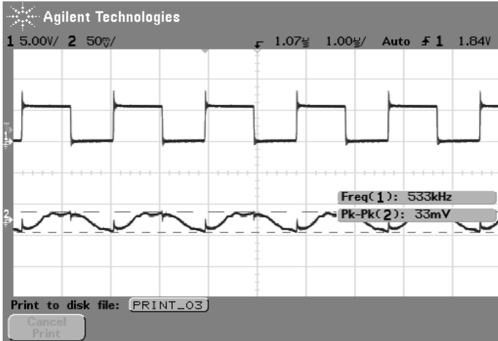
Figure 3. Typical Switch Node and Output Ripple Waveform
