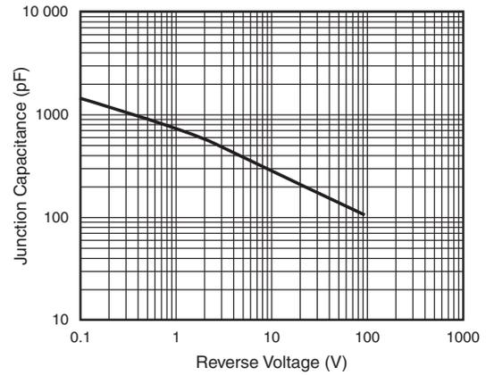
Fig. 4 - Typical Junction Capacitance Per Diode
