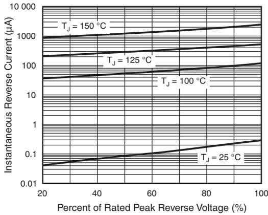
Fig. 3 - Typical Reverse Characteristics Per Diode
