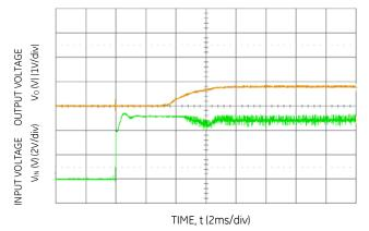
Figure 30. Typical Start-up Using Input Voltage (VIN = VIN, NOM,  $I_0 = I_{0,max}$ ).
