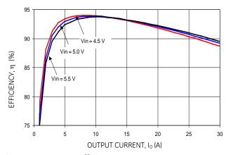
Figure 31. Converter Efficiency versus Output Current.
