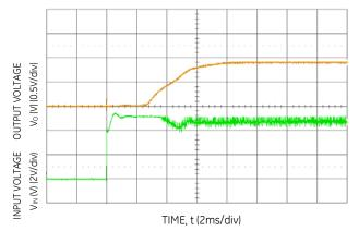
Figure 36. Typical Start-up Using Input Voltage ( $V_{IN} = V_{IN,NOM}$ ,  $I_0 = I_{0,max}$ ).
