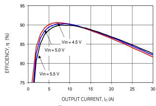
Figure 25. Converter Efficiency versus Output Current.
