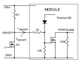
Figure 50. Remote On/Off Implementation using ON/OFF.
