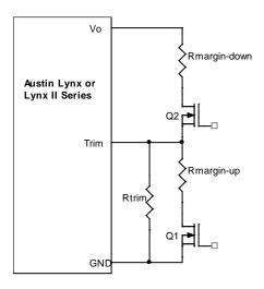
Figure 53. Circuit Configuration for margining Output voltage.
