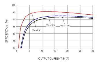
Figure 16. Converter Efficiency versus Output Current.
