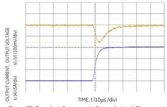
Figure 27. Transient Response to Dynamic Load Change from 0% to 50% of full load with  $V_{\text{IN}}$  =5V.
