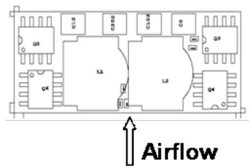
Figure 55. Airflow direction for thermal testing.
