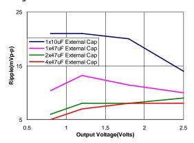
Figure 49. Output ripple voltage for various output voltages with external  $1x10 \mu F$ ,  $1x47 \mu F$ ,  $2x47 \mu F$  or  $4x47 \mu F$
