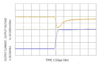
Figure 33. Transient Response to Dynamic Load Change from 0% to 50% of full load with  $V_{\rm IN}$  =5V.
