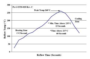
Figure 60. Recommended linear reflow profile using Sn/Ag/Cu solder
