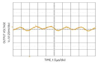
Figure 32. Typical output ripple and noise (VIN = VIN,NOM,  $I_0$  =  $I_{0,max}$ ).
