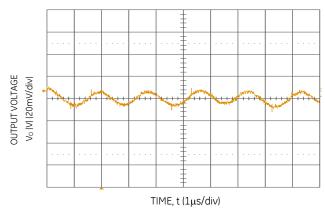
Figure 26. Typical output ripple and noise ( $V_{IN} = V_{IN,NOM}$ ,  $I_0 =$ lo,max).
