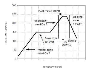
Figure 58. Reflow Profile for Tin/Lead (Sn/Pb) process.
