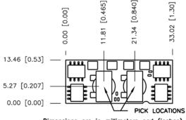
Dimensions are in millimeters and (inches).
