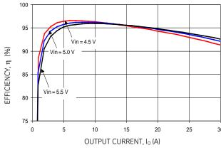
Figure 37. Converter Efficiency versus Output Current.
