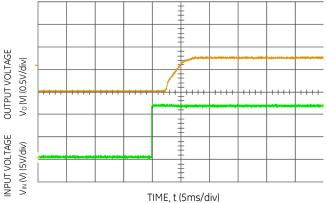
Figure 3. Transient Response to Dynamic Load Change from 0% to 50% to 0% of full load with  $V_{\text{IN}}$  =12V.
