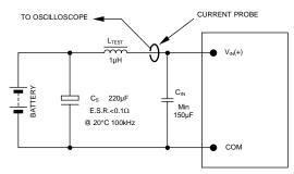
NOTE: Measure input reflected ripple current with a simulated source inductance ( $L_{TEST}$ ) of 1 $\mu$ H. Capacitor  $C_S$  offsets possible battery impedance. Measure current as shown above
