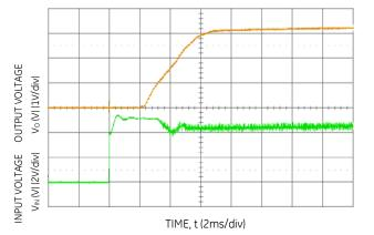
Figure 39. Transient Response to Dynamic Load Change from 0% to 50% of full load with  $V_{\rm IN}$  =5V.
