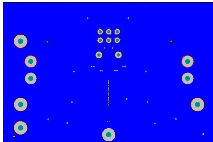
Figure 2. PCB Copper Layout & Silk Screen – Bottom
